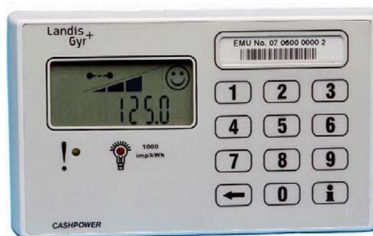
Figure 2: Customer Interface Unit
