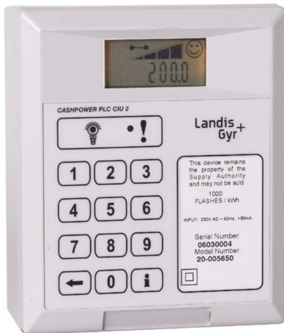
Figure 2: PLC Customer Interface Unit
